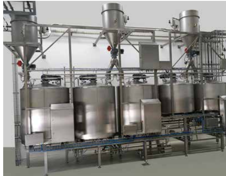
Pre-dough system in a large bakery.
